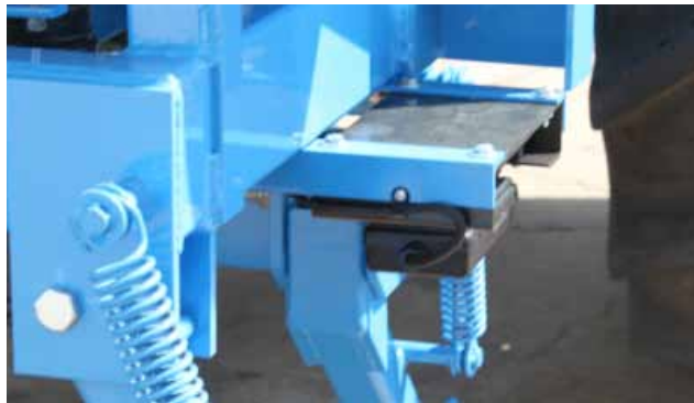
Radar Sensor *as viewed from the rear, lower right side of the machine
