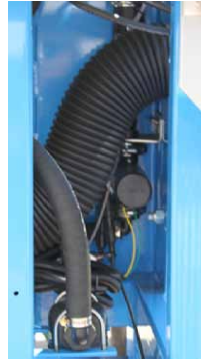
Control Valve/Flow Meter Assembly *as viewed from the rear of the machine with the back panel removed
