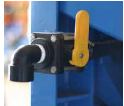
Main tank dump valve
