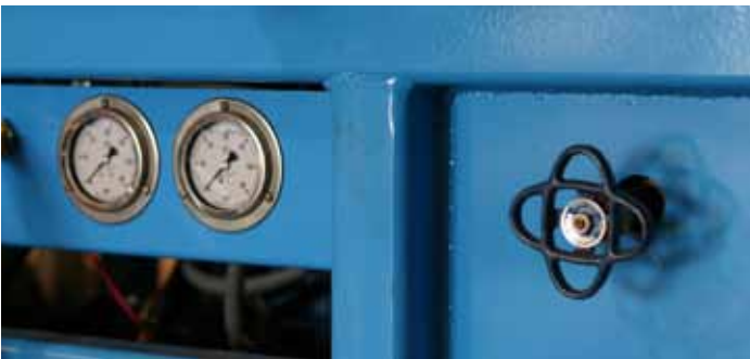
P/N 1039-A: Panel Mount Liquid Pressure Gauge (0 - 60 PSI) P/N 1039: Panel Mount Air Pressure Gauge (0 - 30 PSI) P/N 7851: Liquid Pressure Valve
