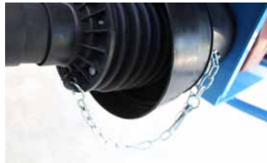
Driveline shield restraint chain installed
