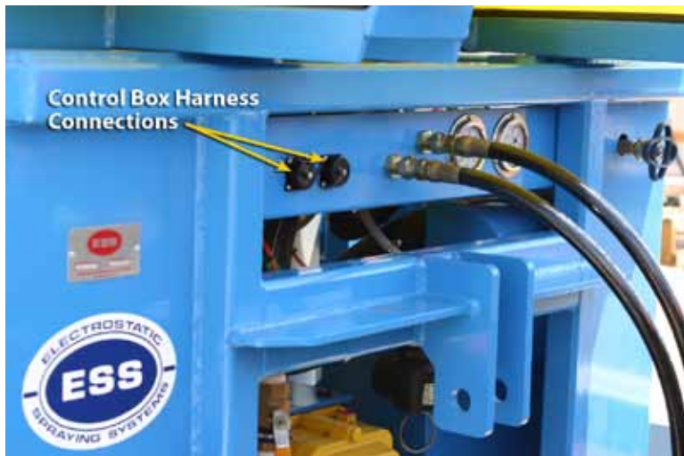
Photograph shows the location of the connections for the Control Box Harness. Remove the caps and attach the harness to the unit.
