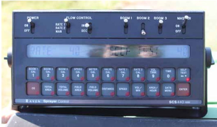
Raven Control Panel
