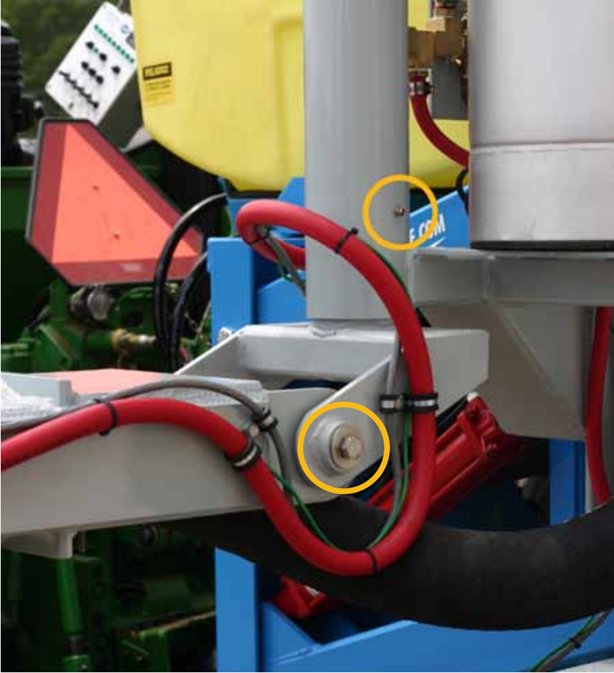
Lubricate swing-arm joints with a lithium-based grease every 8 hours of operation
