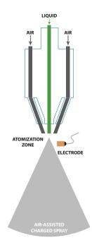
ESS Electrostatic Sprayers use electrostatic technology to give superior spray coverage. But just what is "electrostatic" technology?
