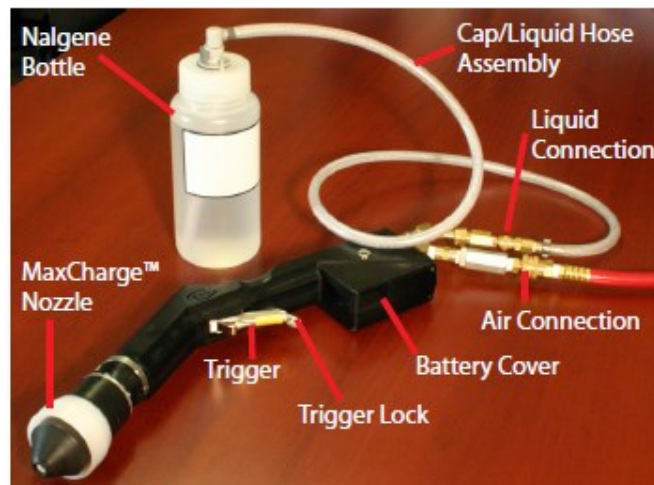
Spraywand Connections
