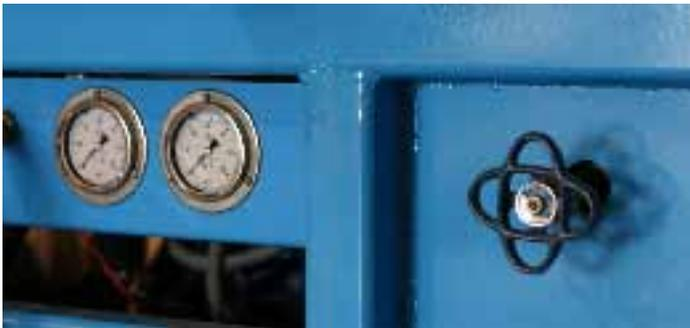
P/N 1039-A: Panel Mount Liquid Pressure Gauge (0 – 60 PSI)
