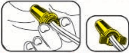
3. Separate connector, removing plastic "link" or "leg" from inner sleeve. Push inner sleeve into pre-filled outer sleeve until double-locked. Ensure that bending sleeve does not come down over either latch. Pre-filled silicone fully waterproofs the connection. Do not reuse.
