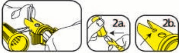
2. Insert wires through flexible sealing fingers and bend bare wire ends together into one "V-Channel." When connecting heavy solid wires, use bending sleeve / depth gauge on outer sleeve of connector (see illustration 2a). For larger connections (e.g. three #12 wires, or equivalent, or more), bend wires into the V-Channel with round hole at bottom (see illustration 2b); pull folded group of wires downward into this hole at bottom of "V."
