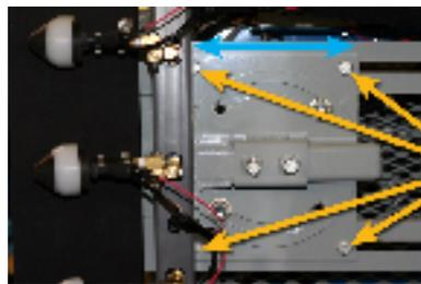
Loosen to slide rotating plate mounting plate
