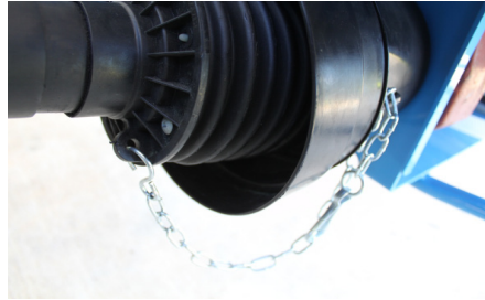
Driveline shield restraint chain installed
