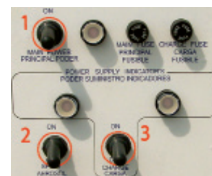
Correct sequence for turning on the Sprayer controls.
