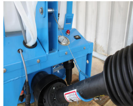
Driveline holding cable
