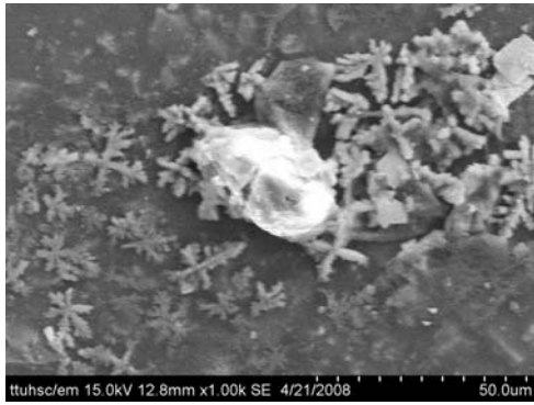
Figure 4.11. Scanning electron micrograph showing Listeria monocytogenes biofilm formed on FRP treated with quaternary ammonium via air pressure sprayer. Magnification was at 1.0 k.
