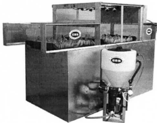
Fig. 3. Electrostatic spray chamber for postharvest application of protective sprays onto fruits and vegetables.
